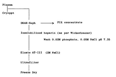
Albumin was added to 4 batches prior to freeze drying but appeared to have no effect. None of the batches were heat treated to inactivate hepatitis virus(es).
